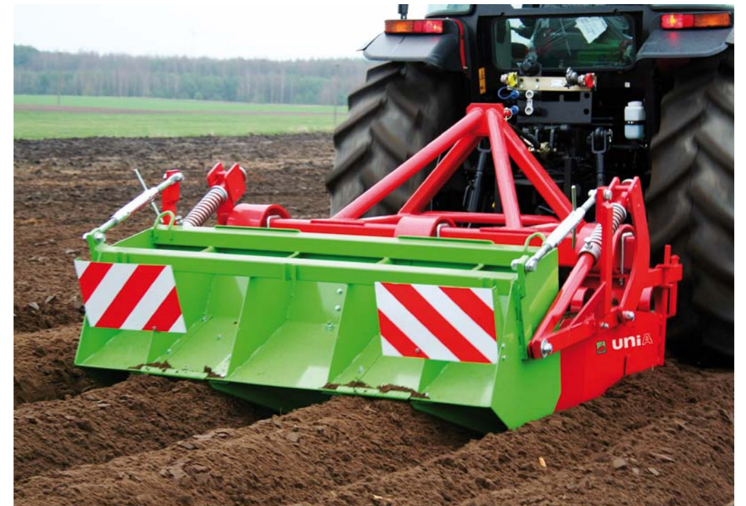
FORMA 2/4 are listers (version 2- or 4-row) with a forming device that enables to obtain a trapezoidal shape of ridges. The inter row width can be adjusted: 70 or 75 cm
