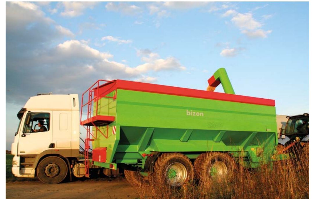
Highly elevated unloading tube enables to reload grains into the trailers of trucks
