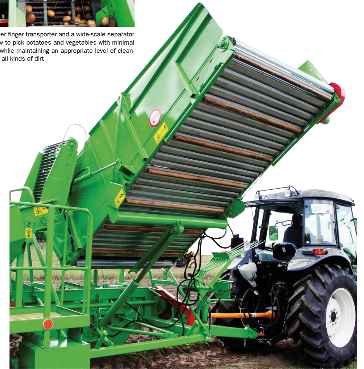
PYRA 3000 combine harvester has a hydraulically elevated tank that enables to unload yield onto the height of up to 3.7 m and PYRA 1600 combine harvester has a tank that enables to unload yield onto the height of up to 2,7m
