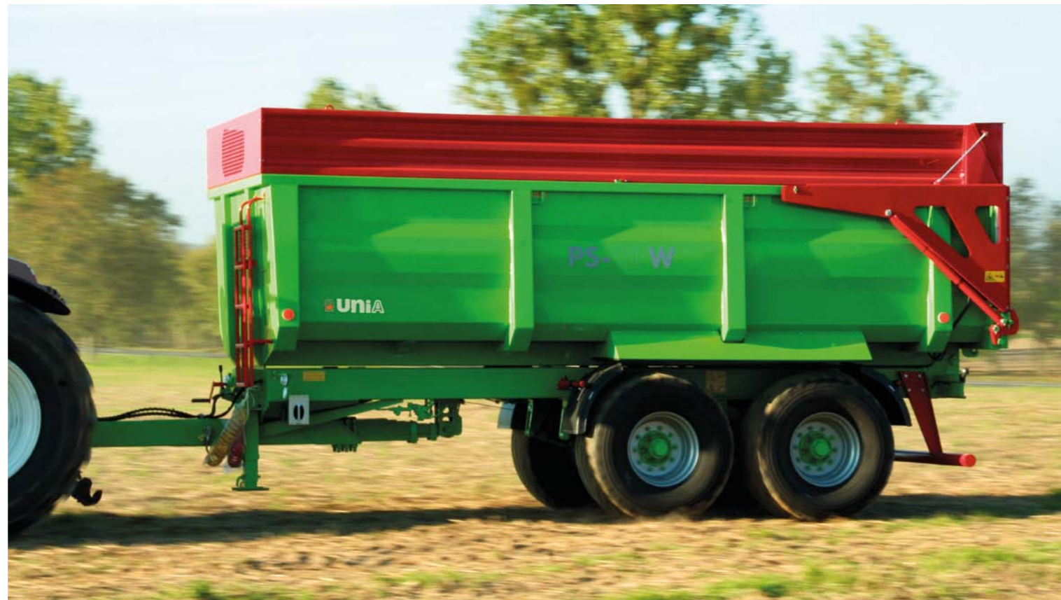
Driving axles of ADR / ATW TUV-approved permit to drive at a speed of 40 km/h
