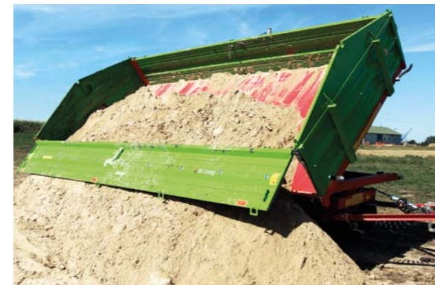
P long – built to transport heavy loads (from sand to stones) Technical loading capacity of the trailer P14 long is 14 000 kg
