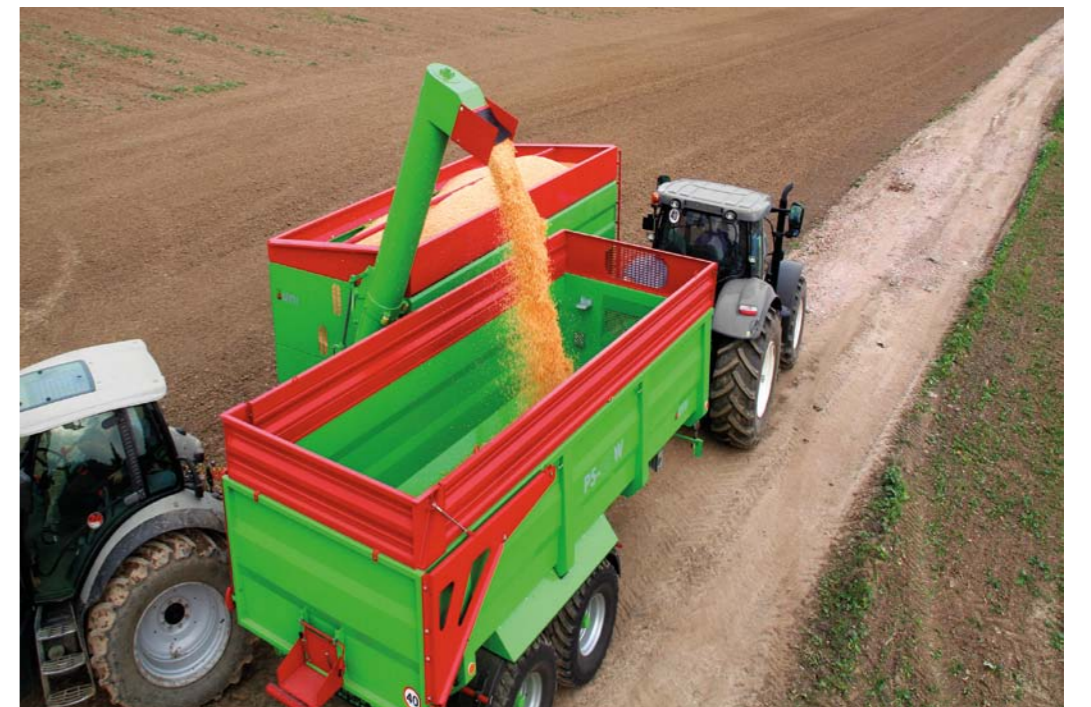
Reloading efficiency is, depending on the material, up to 200-400 t/h
