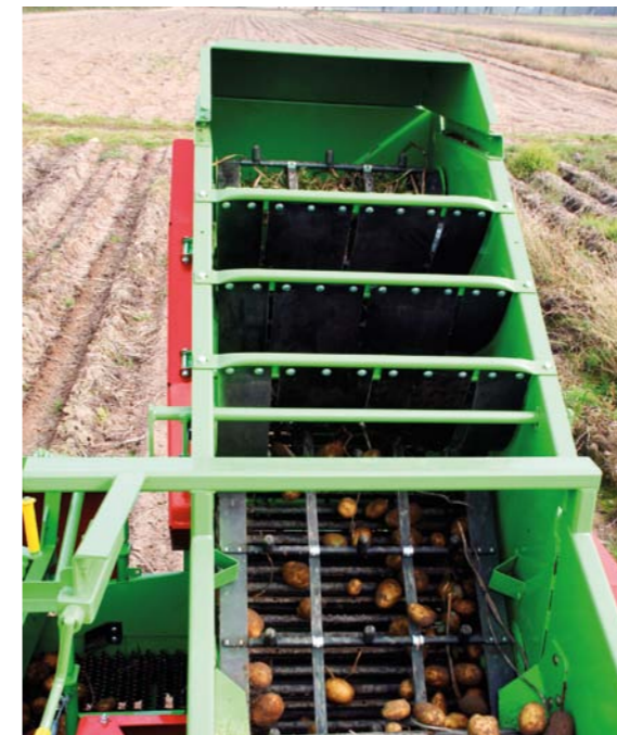
Adjusted rubber finger transporter and a wide-scale separator of haulm allow to pick potatoes and vegetables with minimal damage rate while maintaining an appropriate level of cleaning of yield of all kinds of dirt
