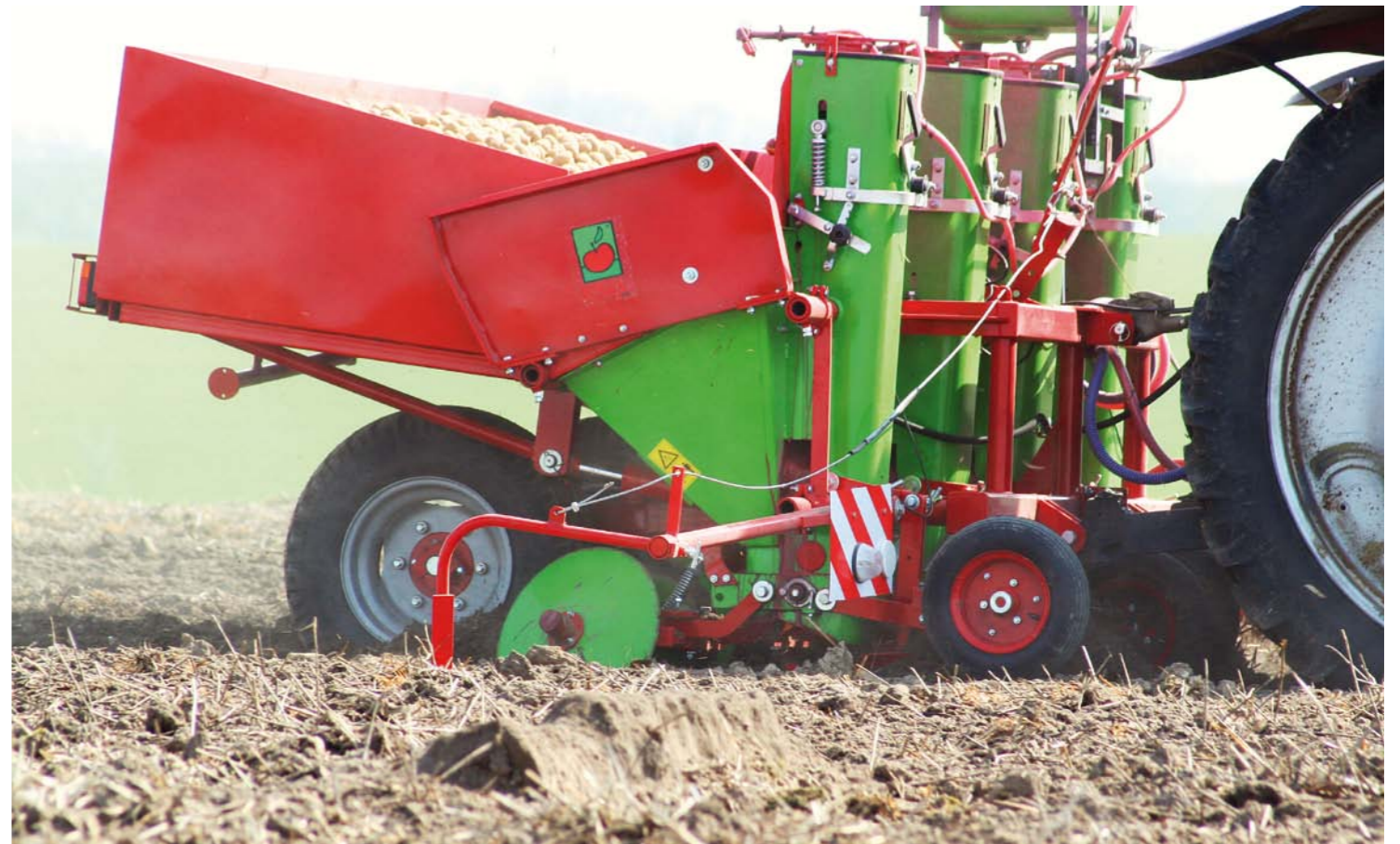
Four-row planter, suspended, for potatoes with an elevated tank that is elevated hydraulically of the capacity of 1100/1150 kg
