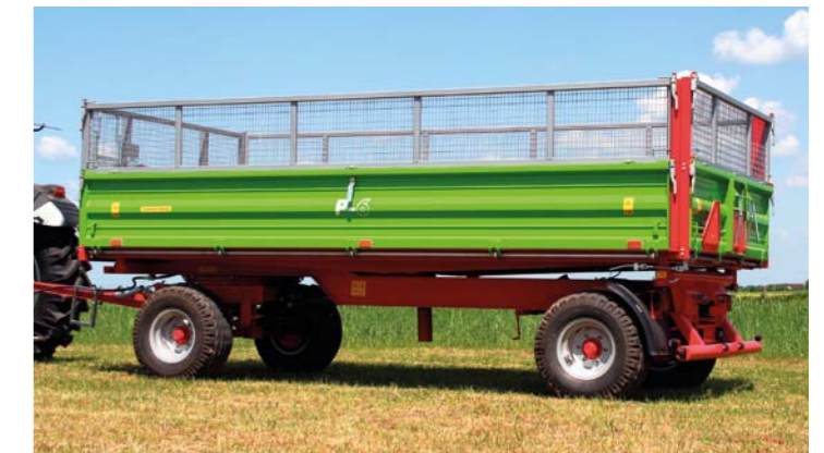
P long – built to transport bulk materials (of chopped corn to dried forage). Mesh top increasing capacity by the height of 1000 mm increase the loading capacity of the P6 long trailer to 20 m 3
