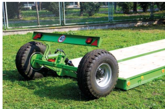
Hydraulically lowered floor of PL 6 platform to the ground level enables to easily load machines
