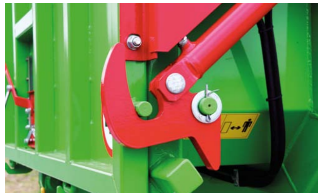
Automatic pressure hooks block the wall on the left after it is lowered, which translates into a super-leakproofness of the box
