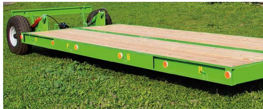
On the left and right side, there are 4 handles to fix belts that secure the transported load
