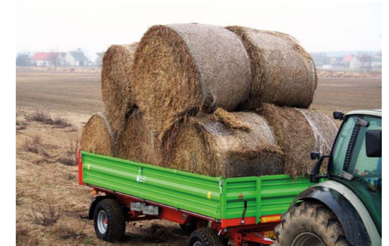
P long – built to transport bales of straw (it's possible to load up to 12 bales of the diameter 120 cm). The length of the load box is 5.25 m, and its width 2.42 m
