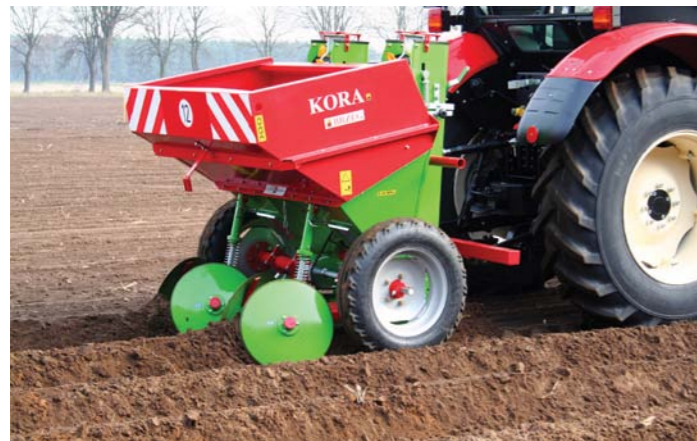
Classic two-row planter with a tank of the capacity 400/450 kg
