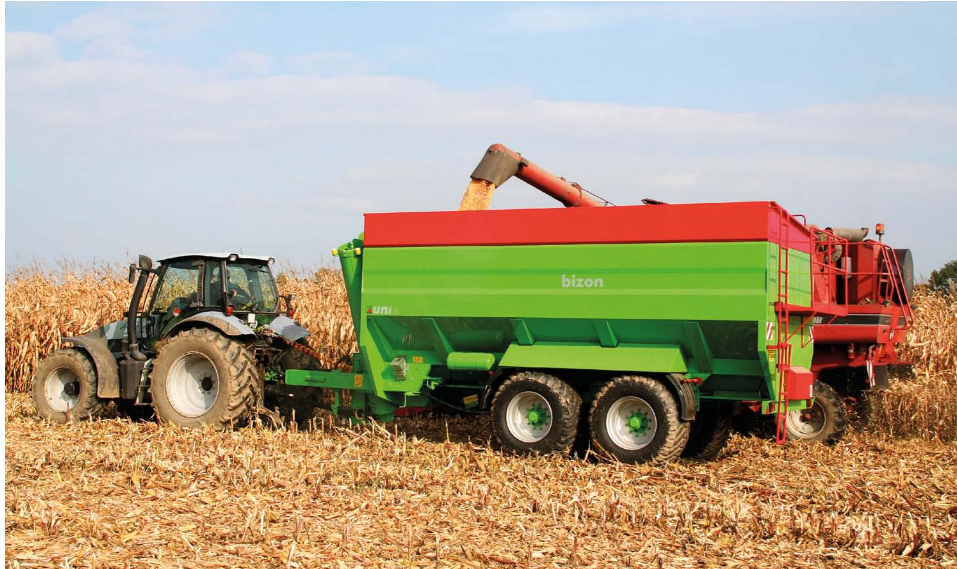
BIZON trailers are attached to a tractor, which makes an efficient set that combines combine harvesters with z transport sets standing on hardened surfaces on the borders of the fields
