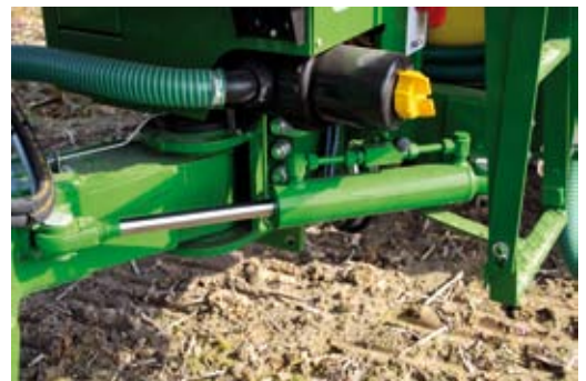
Twisting drawbar for easy manoeuvring following the marks of tractor wheels
