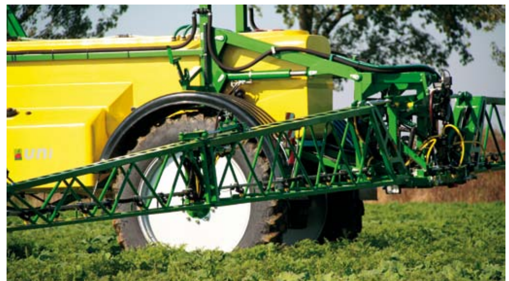
Suspension of the beam on the parallelogram with two hydraulic cylinders and hydraulic shock-absorber eliminates free movement of the beam and allows it to raise up to 2.5 m
