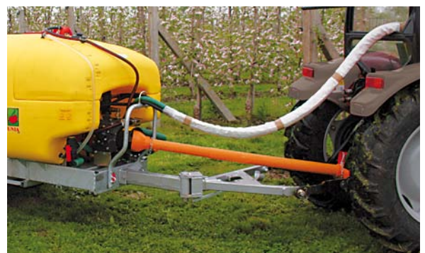
Twisting drawbar for easy manoeuvring following the marks of tractor wheels
