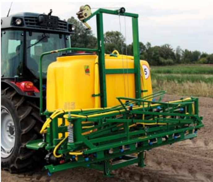
EKO – the field beam is unfolded, folded or lifted manually. Lifting is aided by a self-locking mechanism protecting the beam against going down suddenly
