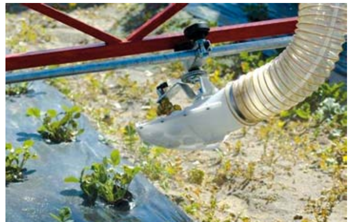
Diffusers are mounted loose on the field boom, allowing to tailor their configuration to individual user's needs
