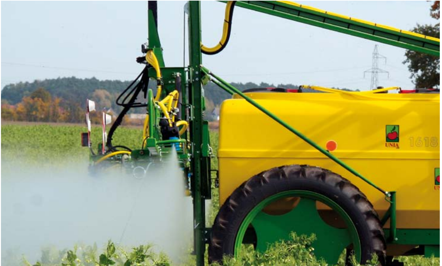
Durable and functional field beams with a tiltable last segment
