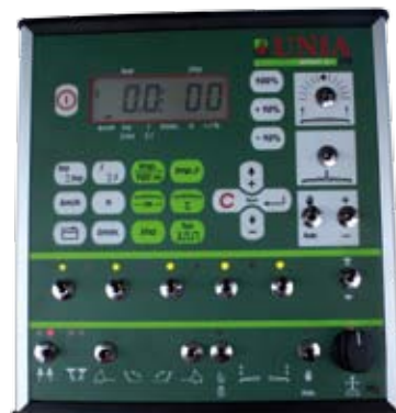
SPRAY computer that controls sprayer operation
