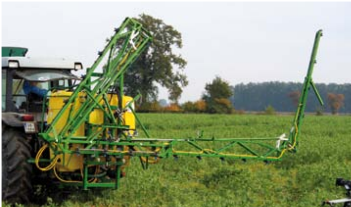
LUX – comfort operation due to a hydraulically folded and unfolded beam
