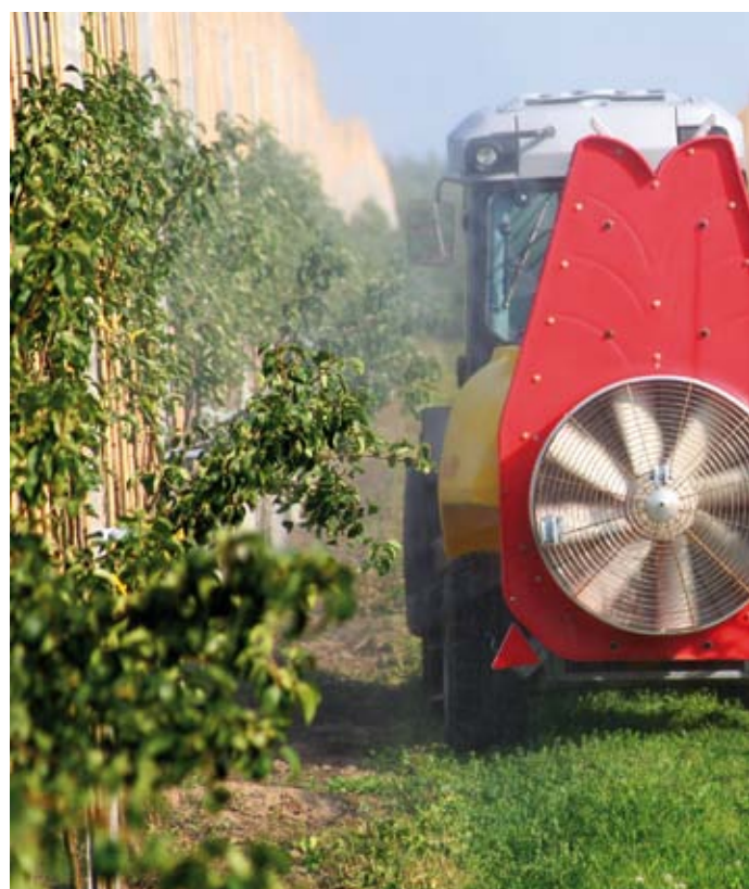
DUET column accessory (two counter-rotating and coaxial rotors) of the max. capacity of 43000 capacity and a range up to 5.0 m, for high planting
