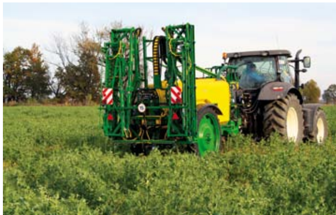
The field beam folded behind the spraying machine (REX type) is available for PLUS spraying machines with tanks 2000 l & 2500 l
