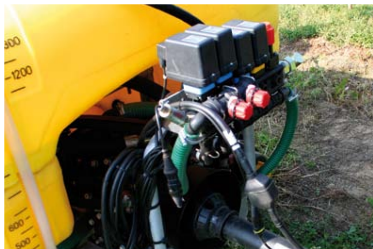
Electrovalve with electronic display of pressure
