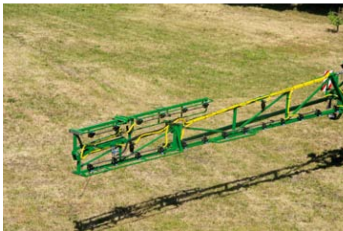
R-system – reduction of the working width of the sprayer: 28/21 m, 27/21 m, 24/18 m, 21/15 m, 18/12 m
