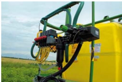
Electro valve that controls the performance of the field beam section
