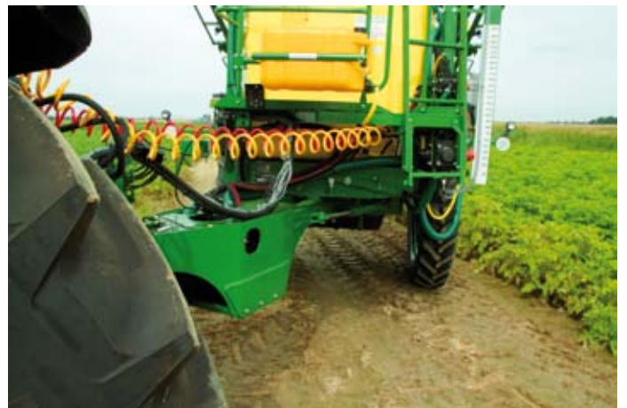
Copying of the tractor tracks by the spraying machine wheels is controlled by SPRAY or UTS computer with a gyroscope sensors system (TRIAL CONTROL)
