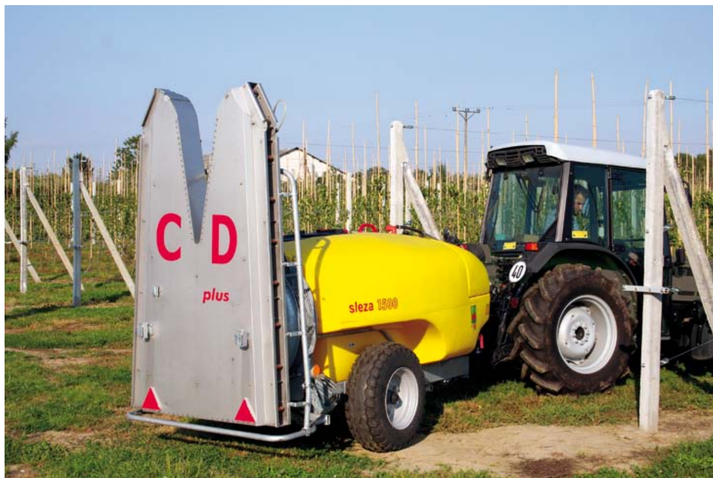
Accessory CD PLUS, of the capacity 45000 m 3 /h and a range up to 4.5 m, for high plantations
