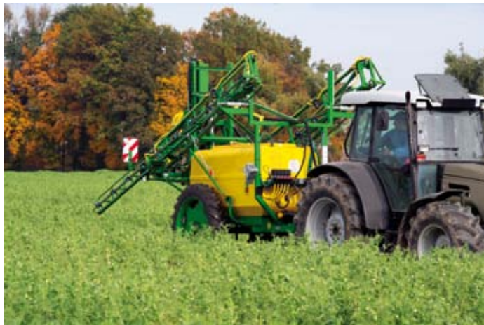
The field beam folded the sides or vertically the spraying machine is available for PLUS spraying machines with tanks 1600, 2000 l & 2500 l
