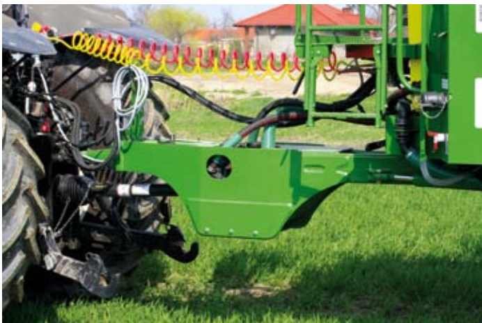
Automatic twisting drawbar for easy manoeuvring following the marks of tractor wheels
