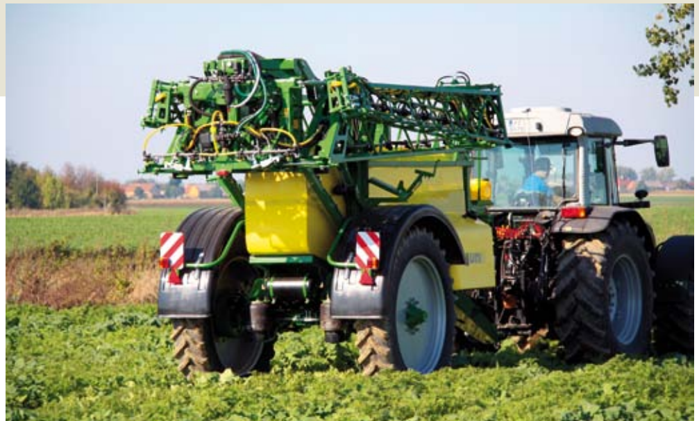
Compact body of the sprayer has 2.8 m of transport width, which makes it possible to transport it on public roads
