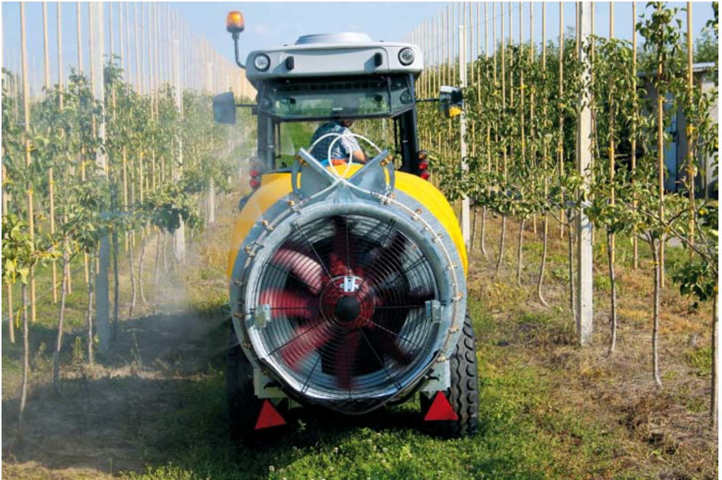
PILMET accessory, Ø 800, of max. capacity of 45000 m 3 /h and a range of 4.5-5.0 m, for traditional cultivation
