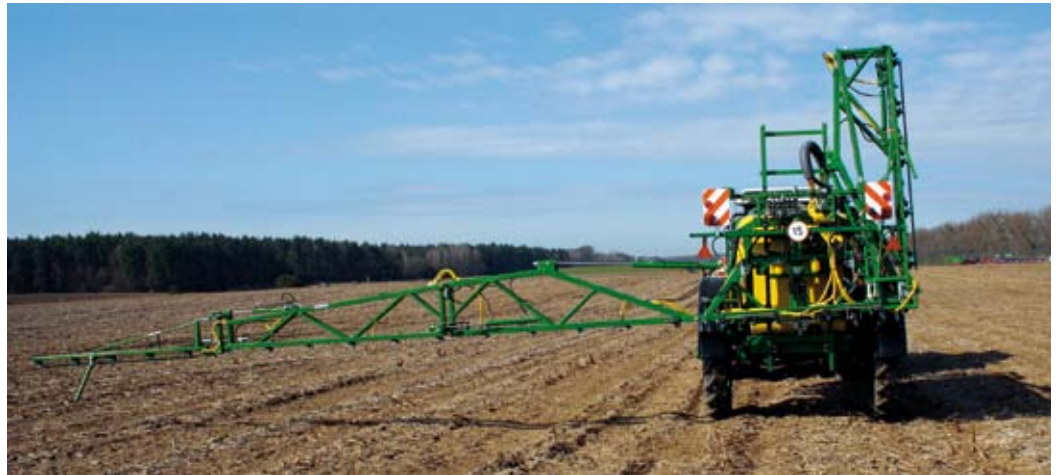
PLUS (REX type) – independently unfolded beams enable omitting obstacles
