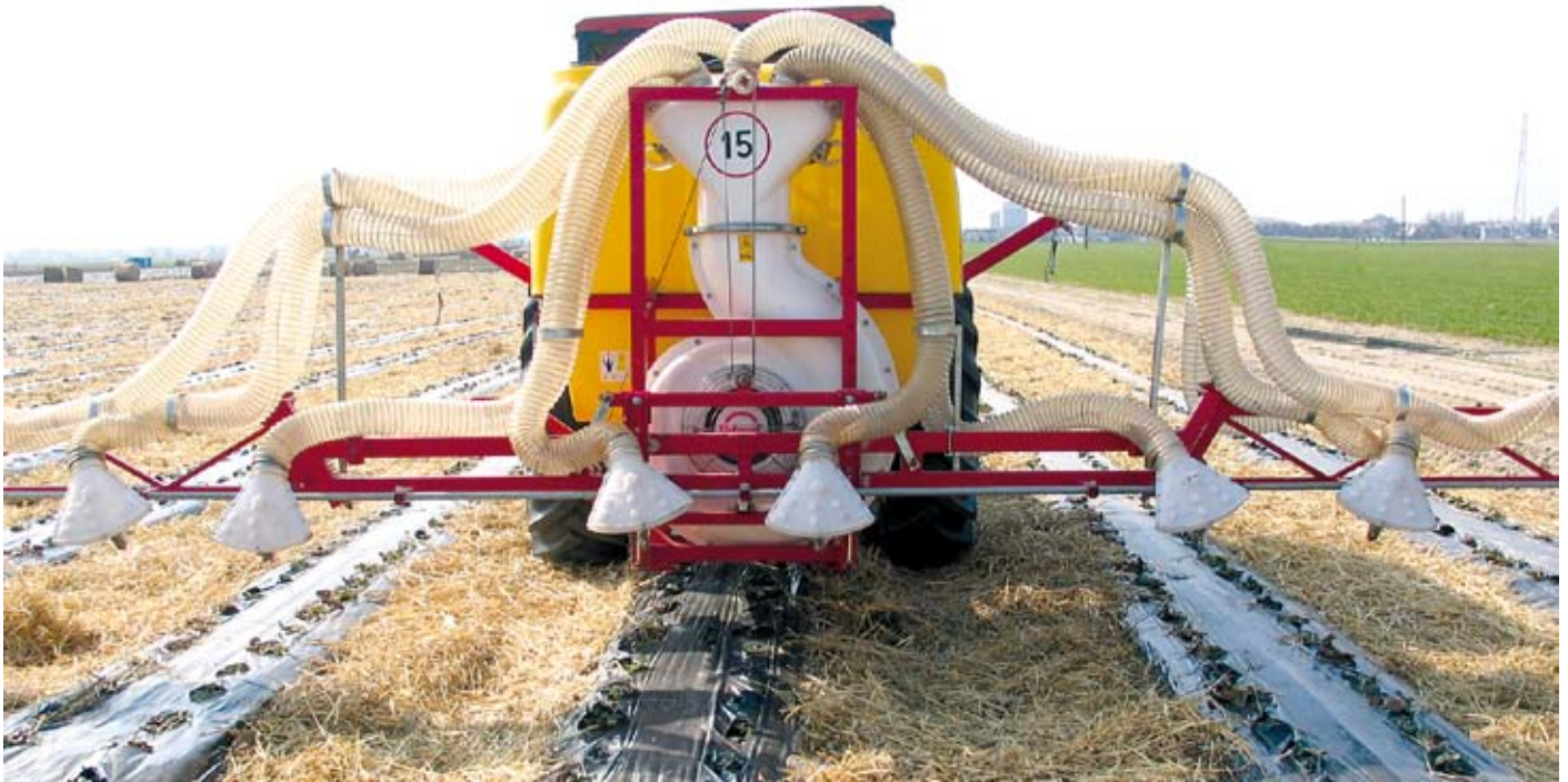
Centrifugal fan, supporting the sprayed stream
