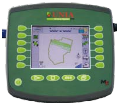
Computer UTS with GPS Track Leader II and Section Control enables the use of precise agriculture benefits
