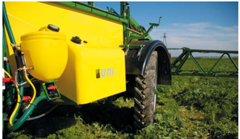
Two tanks situated on both sides for clean water (2x300 l) assure symmetric load of the sprayer frame and provide water to clean the tank
