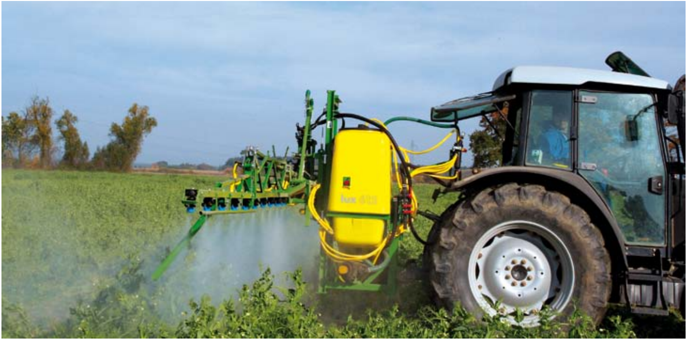
LUX – the whole field beam is made of bent metal sections which results in durability and stiffness
