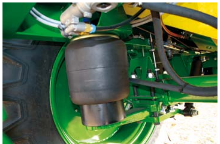
Cushioned axis increases the comfort of work and enhances the durability of the sprayer
