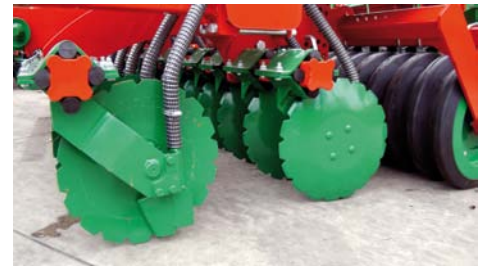
The single disc couler on rubber shock absorber - Pressure of 100 kg, recommended for sowing in technology minimum soil cultivation
