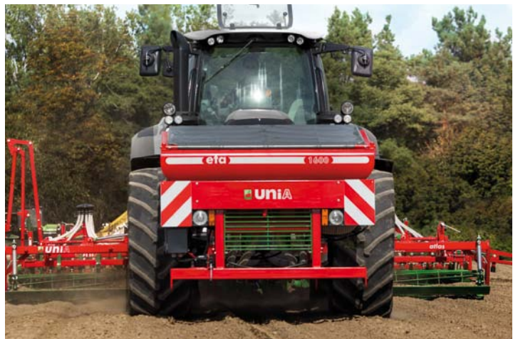
FV 1600 mounted on the 3-pint linkage of the tractor (600 dm 3 possible raiser)
