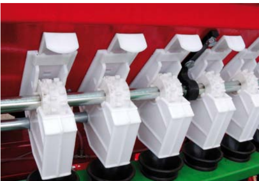
Two piece integrated sowing apparatus (divided wheels to fine and coarse seed)
