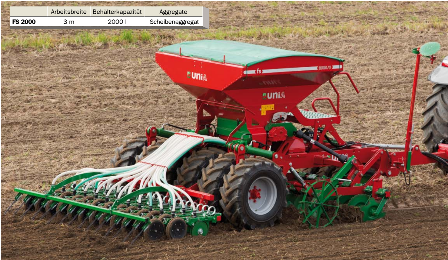
Tire roller with a diameter of 1100 mm = stabile work under all conditions
