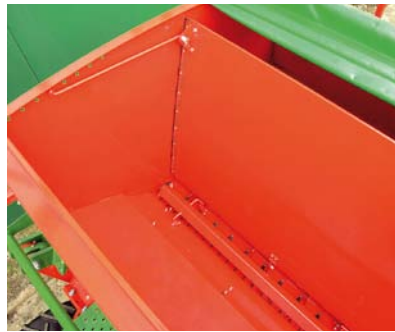
AMBER DUPLO in addition to the sowing apparatus is equipped with apparatus sowing fertilizer and fertilizer-divided seeding hopper
