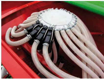
Electrovalves mounted on sowing lines make easier to place process paths.
