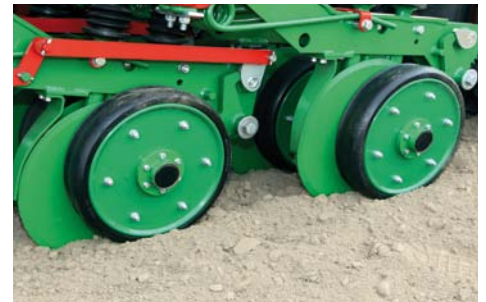
The double disc couler with copying wheel - pressure 40 kg / couler, provides a copy area. Recommended for sowing in a traditional soil cultivation
