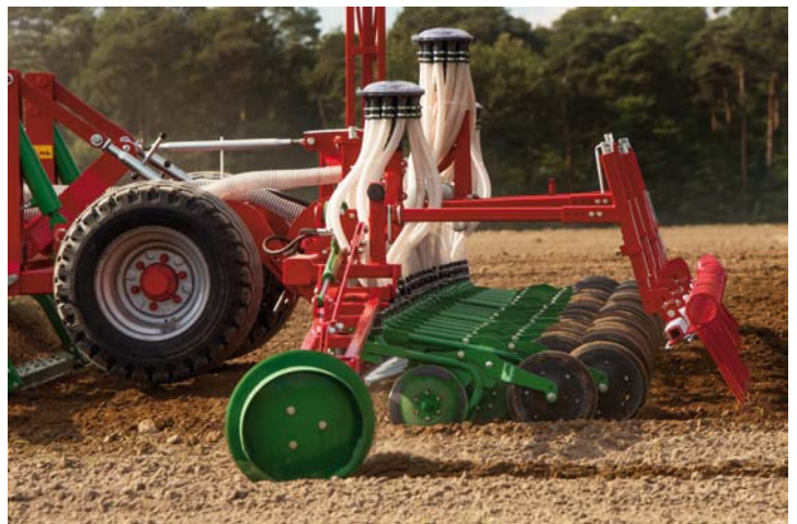
Seed beam with a width of 6 m coulter, light (pressure 25 kg / coulter)
