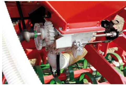
Sowing apparatus can dose seed thick or fine grain in the range 1,8 - 400 kg/ha
