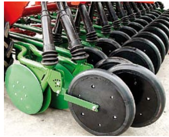
Double disc coulters alternating self-cleaning with pressing-copying wheels
