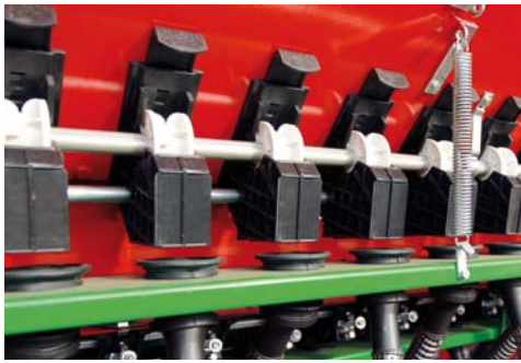
AMBER DUPLO in addition to the sowing apparatus is equipped with apparatus sowing fertilizer and fertilizer-divided seeding hopper
