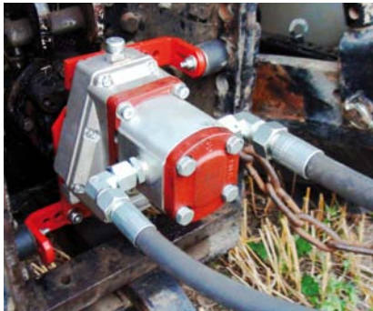
Hydraulic pump with the capacity 30 l/ min. Powered by tractor's PTO shaft
