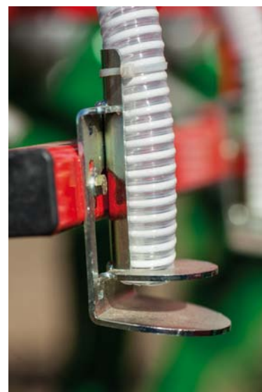
Seeds hit the diffusion plate, which increases the width of the sowing
