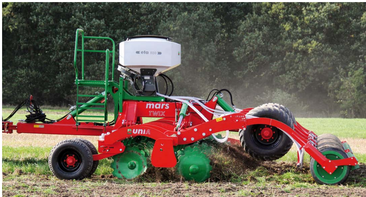
Dispenser drill ETA – you can sow small seeds of plants aftercrop and grasses
