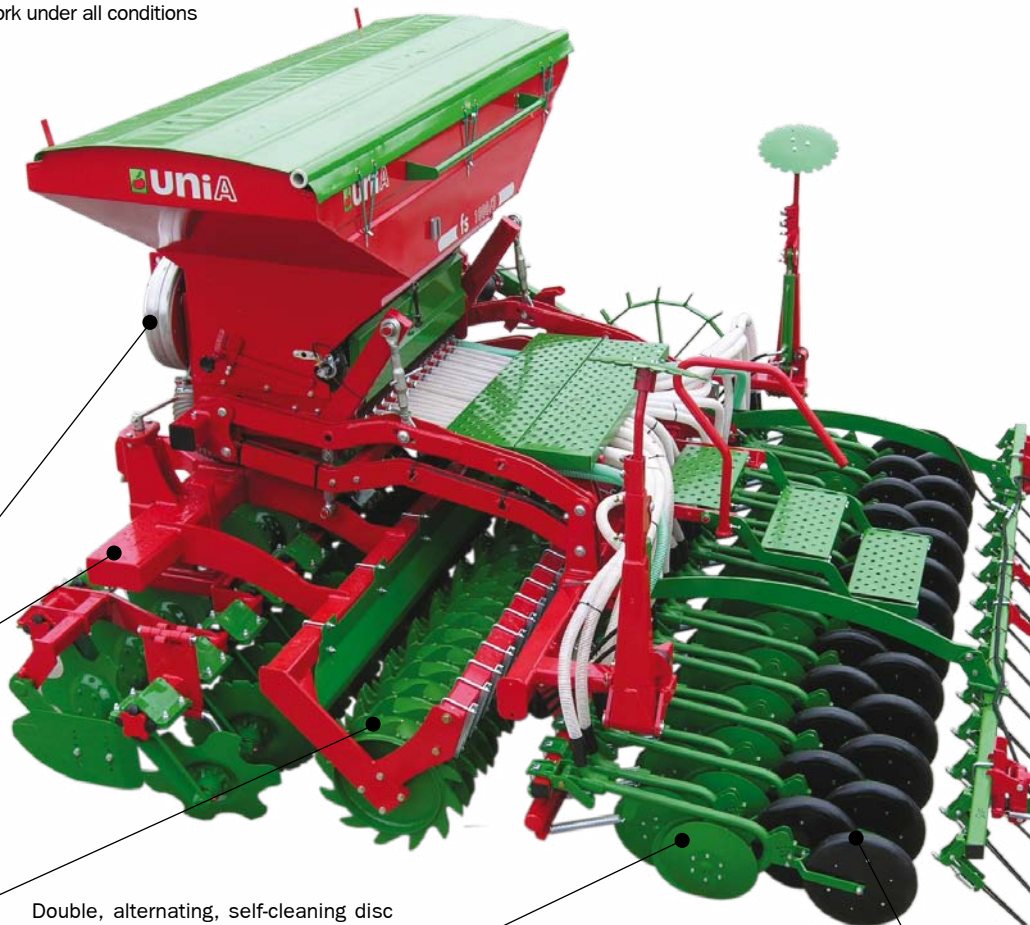
Pressing and copying unit ensures appropriate seed to soil contact and maintains the desired seeding depth in all conditions.
