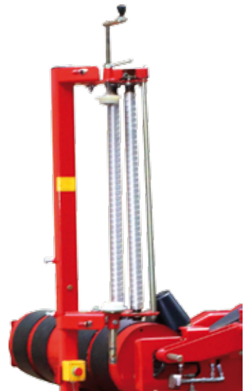
Foil feeder - supports the film 500 and 750 mm
