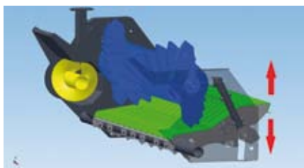
Transport rotor – relates to the balers without cutting system
