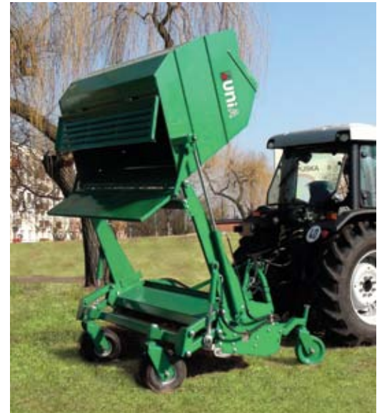
KORNİK Combo with a container lifted up to 1.7 m – ideal for works in parks, city green zones, etc.
