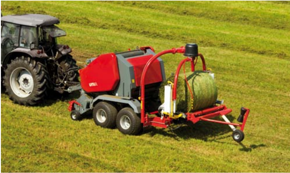
Bale transfer and wrapping is done in automatic mode
