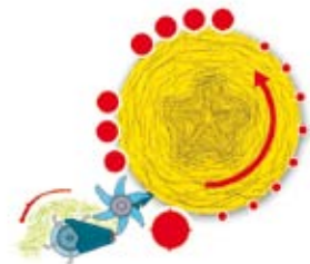
DF 1,8V / 1,8Vd chamber with chains and rollers
