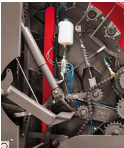
Automatic chain lubrication – comfort and convenience
