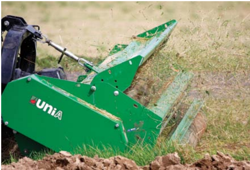
The KORNİK flail mowers may be used for mowing grass and shredding branches at field borders
