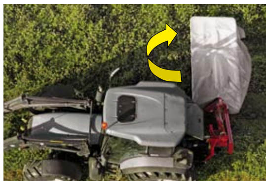
Transport position. Hydraulics in standard
