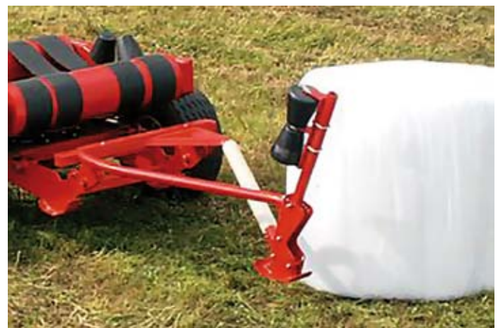
Bale rotator – sets the bale in a vertical position
