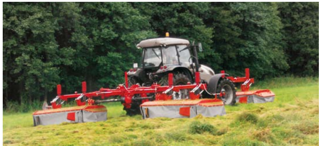
ALKA 3 XL – a set of 3 mowers. Rear mounted mowers on the common frame. Hydraulic folding for transport
