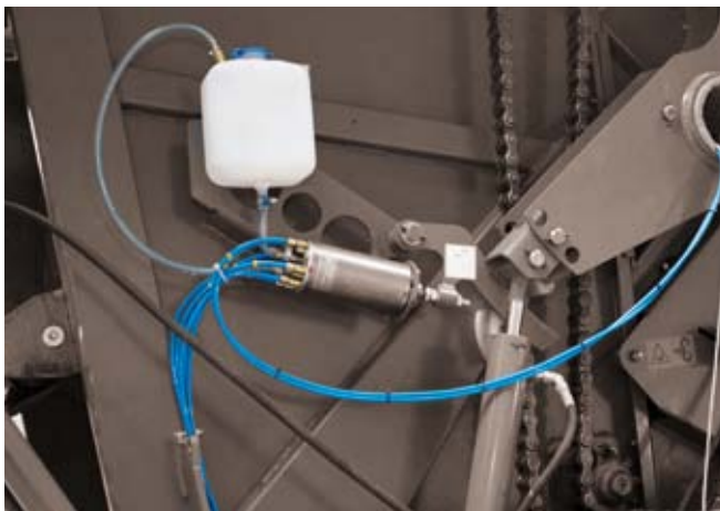
Automatic lubrication – adjustable oil flow to the individual sections
