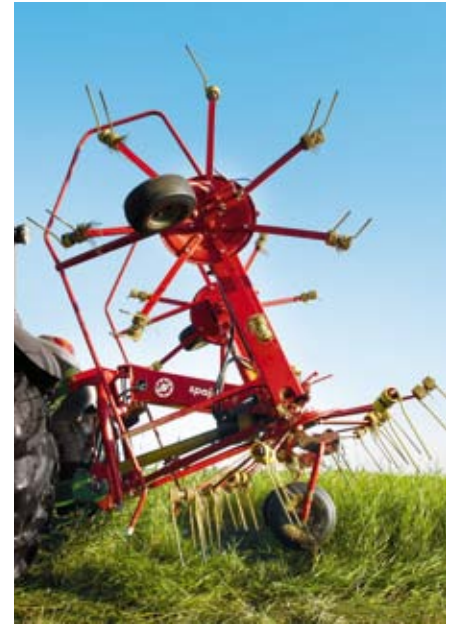
Transport – Outer impellers are folded hydraulically for the transport position
