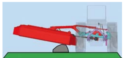
Bump protection saves the mower from damage
