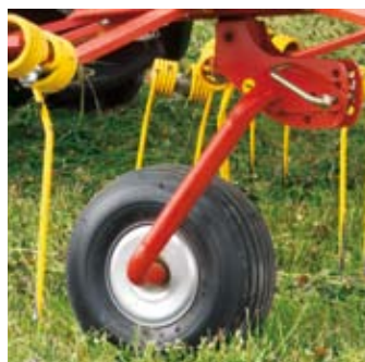
Regulation of scattering angle - Gradual regulation of the scattering angle makes it possible to adjust the machine to the material quality and the working speed
