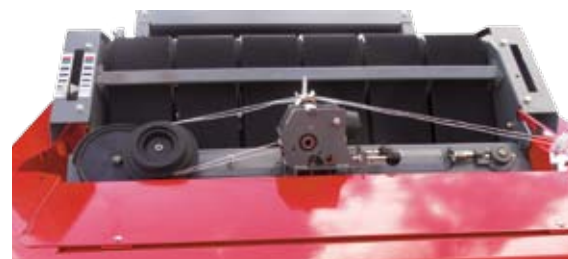
Double twine binding – standard for PP 1,5 | DF 1,8 C
