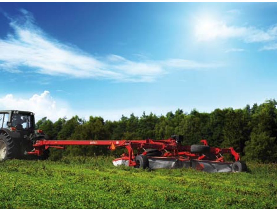
Turbo-drying instead of tedding. Two types of conditioners at choice. Rubber rollers or fingers
