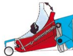
Non stop – individual protection of 14 knives
