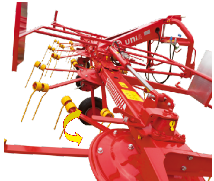
Throwing away of baulk - You can use a lever on the frame to change the position of wheels in order to set the throwing angle to the 'off-the-baulk' mode
