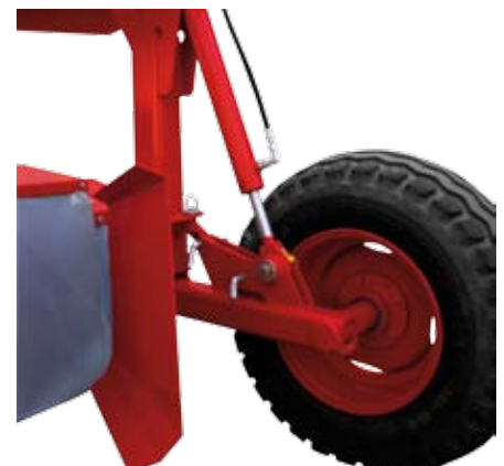
Cutting height adjustment by the bumper and hydraulic cylinders
