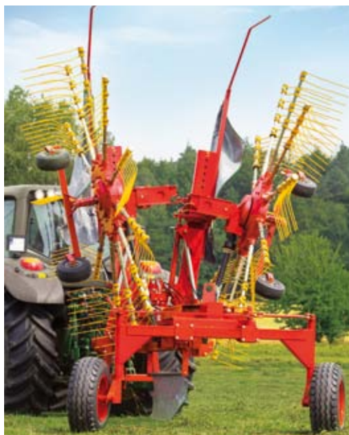
Good manoevrability during U-turns – the wheels are controlled
