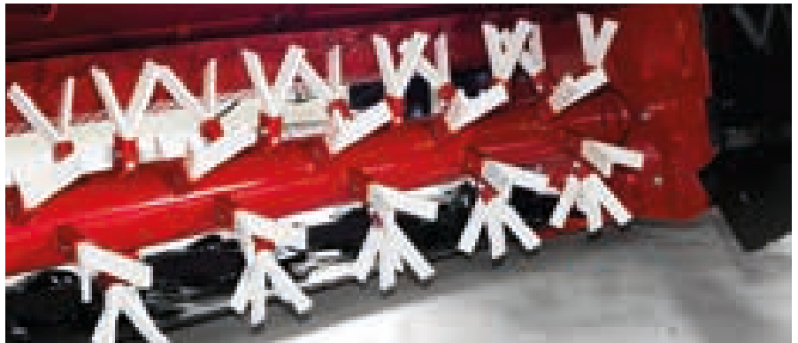
Finger conditioner (FC) with plastic fingers and the possibility of setting the intensity of conditioning offer optimum conditioning.
