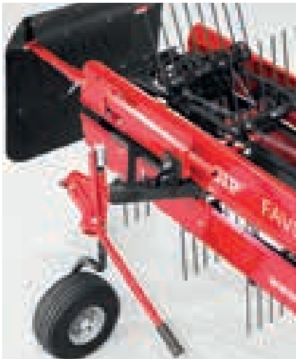
Adjustment of wheel height with lever
