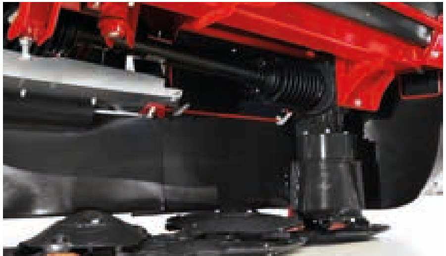
Transmission of power through the PTO shaft and angle gear directly to the first disc
