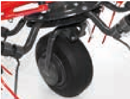
Wheels with multi-level height and spreading angle adjustment. For tedding near the edge of the fields it is possible to shift the wheels.
