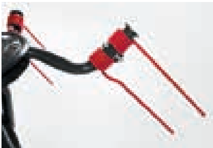
Protection against loss of broken spring tines
