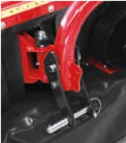
Universal three point linkage for different types of mountain tractors
