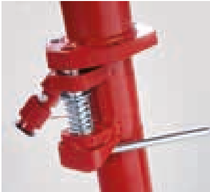
System for rotation of external rotors for a narrower transport width
