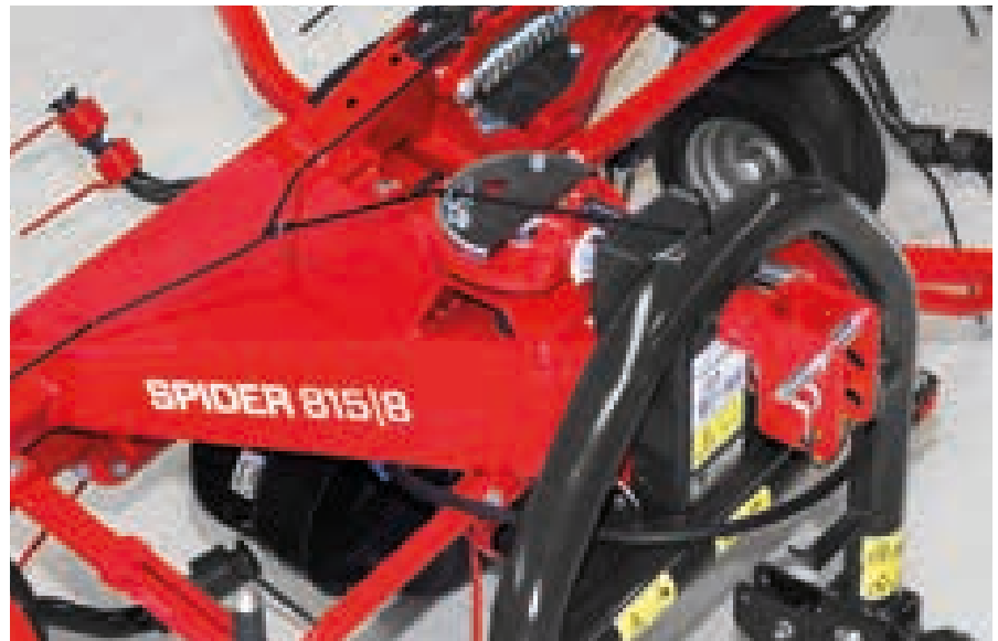
A pivoting linkage allows the machine to follow the tractor easier. In the transport position a special mechanism locks the pivoting linkage perpendicular to the tractor.
