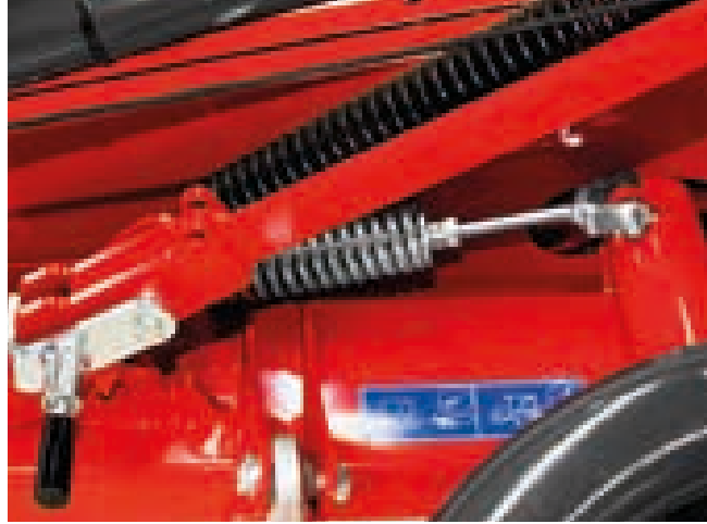
Tensioning spring of the belt drive
