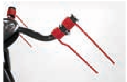
Spring tine arm with protection against loss of broken spring tines
