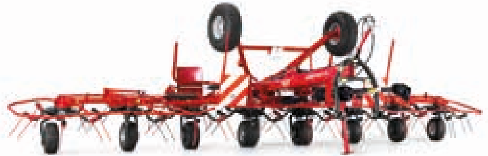
Trailed version of tedder with transport undercarriage
