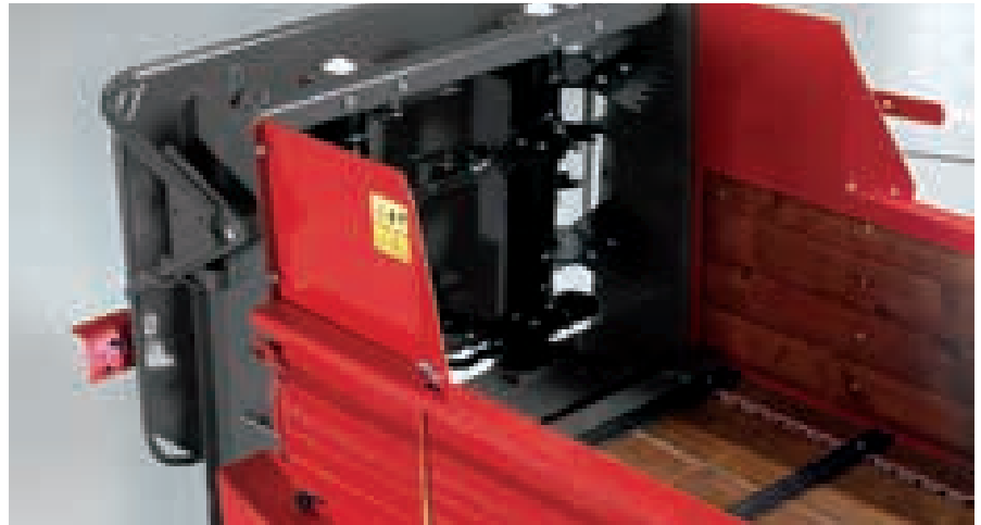
The spreading unit with rear protection (optional) and a pair of vertical beaters (with removable segments) that achieve a fine and even spread.
