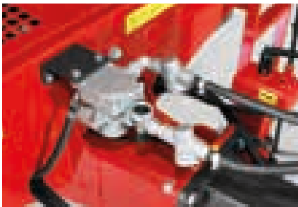
The two-way air brake system with ALB offers increased safety when having to brake when the manure spreader is fully loaded.
