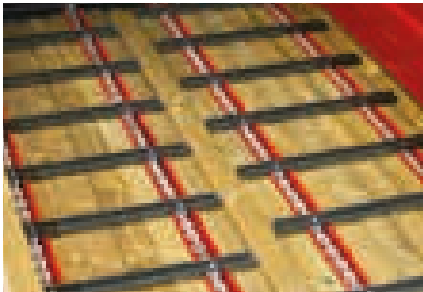
The floor chain conveyor consists of 4 chains dim. 13 x 36 mm and is driven by a hydraulic motor.
