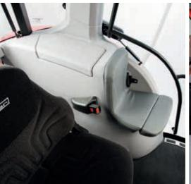
**Comfort for driver and co-driver** Besides the cab suspension, the driver's seat with low-frequency air suspension and the padded passenger's seat ensure comfort when driving.
