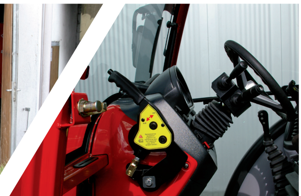
GEOTRAC 94 ep: Safety lock for mountain usage
