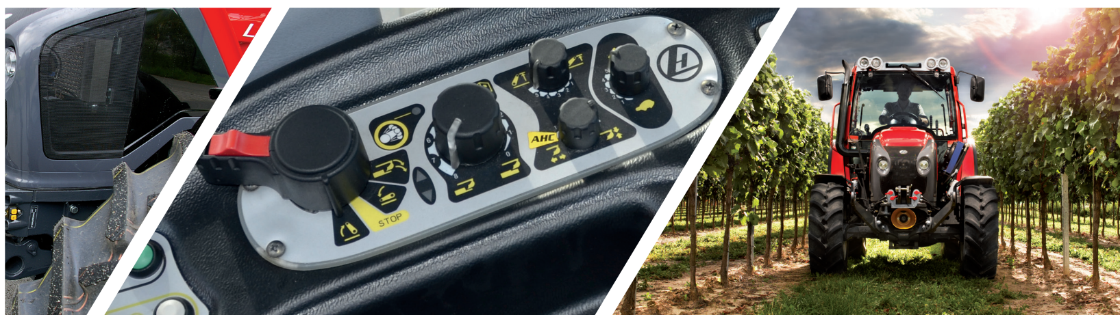
EFH - Electronic front linkage control with vibration damping
